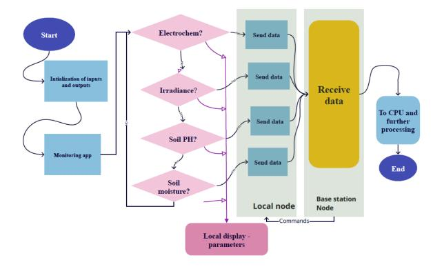
Figure 4: Flow diagram of the initial proposed system
