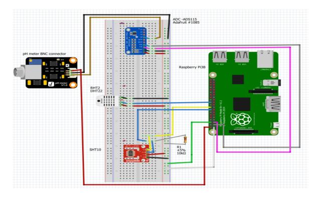
Figure 13: Circuit connections of Prototype 2 designed using fritzing
