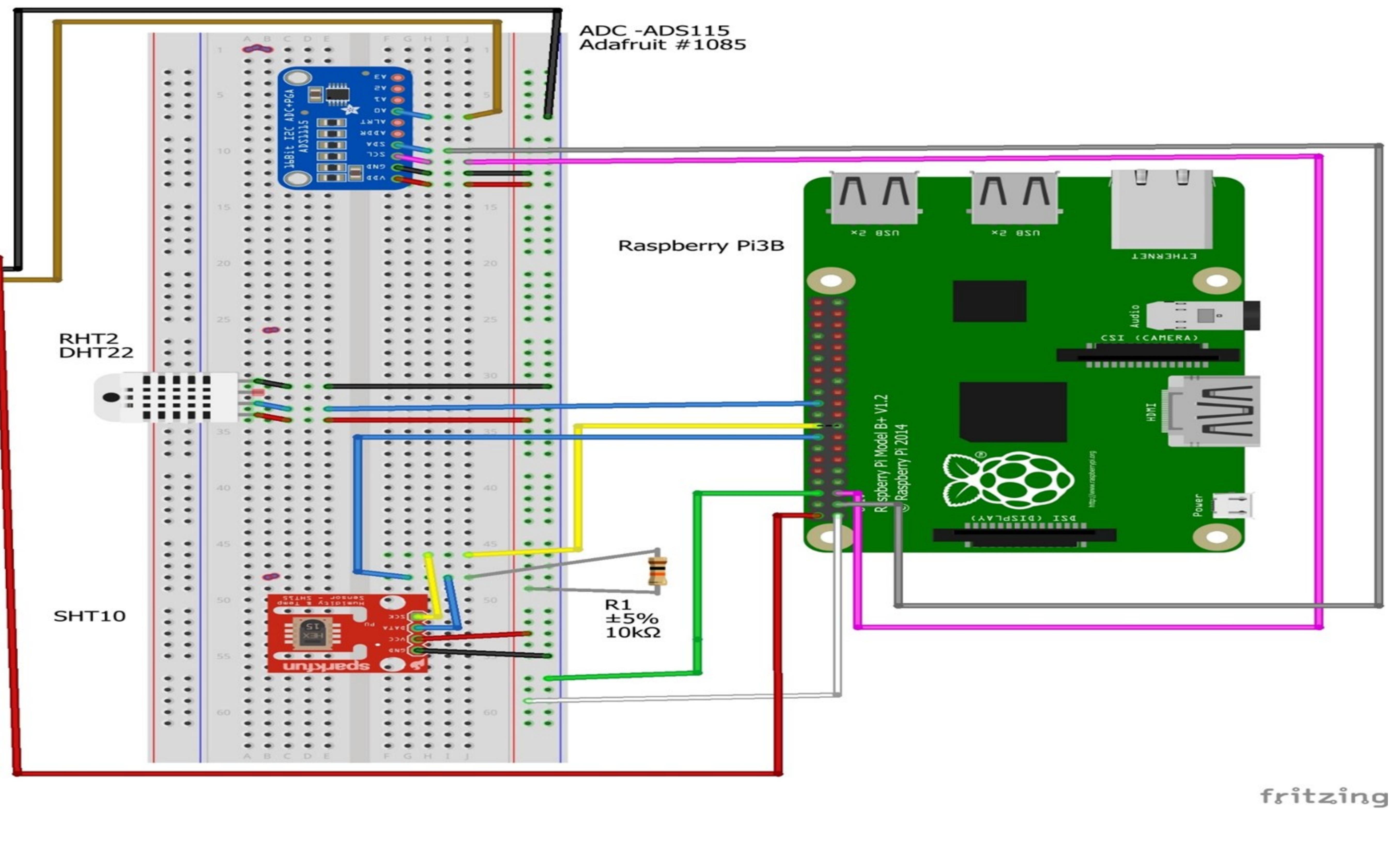
1.System Hardware connection Description. In this study, the probe is connected via ADS 1115 using I2C 2. The SHT10 functions at a range of -200C to 600C hence suitable for use in East African weather. The error/drift is ±4.5%. It has four connections 3.The DHT22 is connected via three pins
