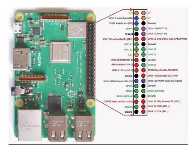
Figure 18: Raspberry pi GPIO pins labelled (eTechnophiles.com, 2021)
