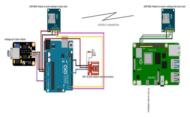
Figure 7: Circuit connections for Prototype 1. Drawn using fritzing software
