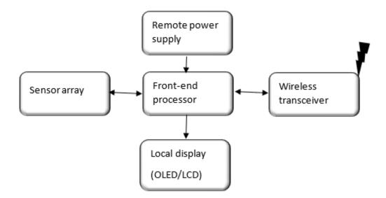
Figure 5: Operation of a local node
