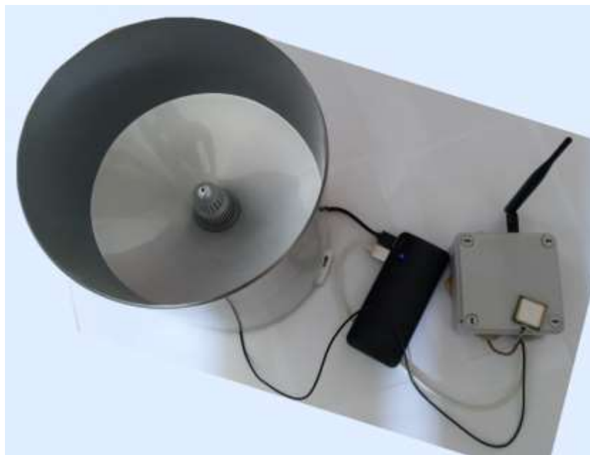
Figure 2: LoRaWAN end device
