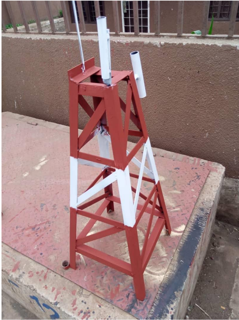
Figure 37: The prototype of the FM broadcasting tower after the welding process
