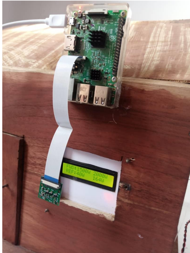
Figure 45: Camera fixed in front of FM transmitter to monitor forward and reflected powers
