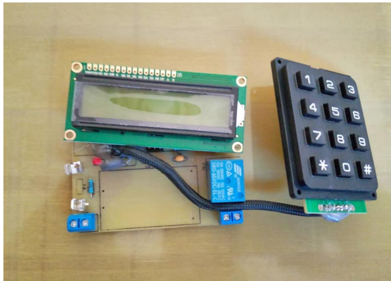
Figure 31: Assembly of the electronic devices after etching and soldering process of energy meter PCB circuit
