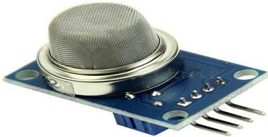
Figure 16: MQ2 Gas Sensor
