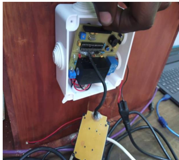
Figure 40: Fixing of embedded systems within the broadcasting room
