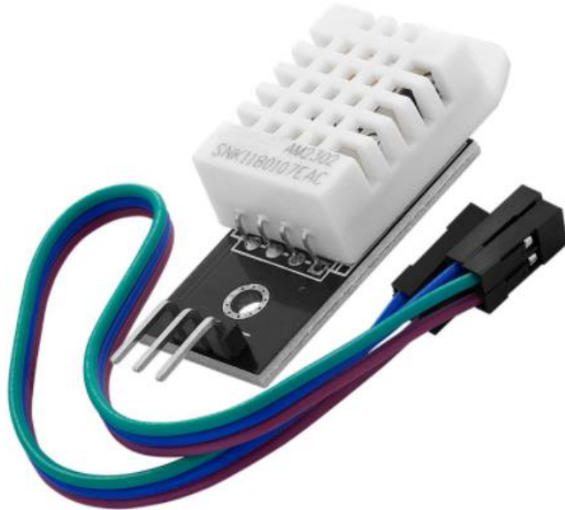
Figure 15: DHT22-Temperature and humidity sensor
