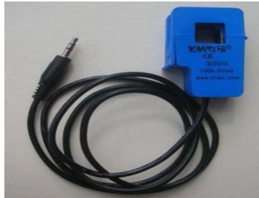
Figure 12: Non-Invasive Current Sensor
