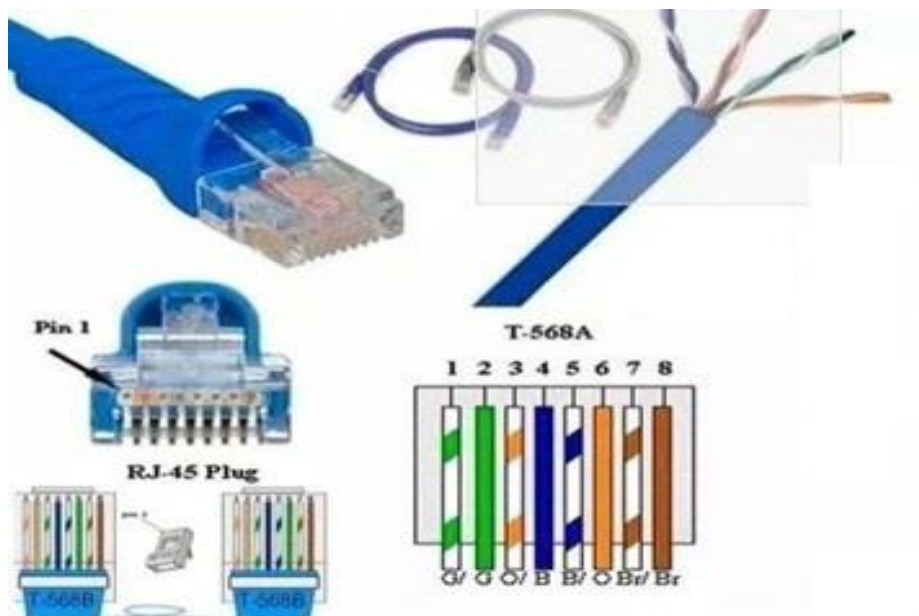
Figure 22: Category 5 Network Cable
