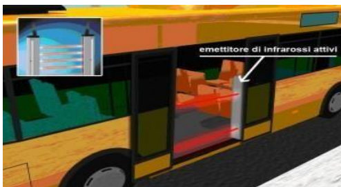
Figure 2: An Installation of Infrared Emitters on Bus Door for Passenger Counting Purposes
