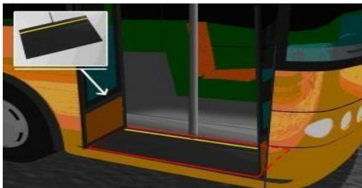
Figure 1: Photo Showing Treadle Mat Sensor Installation on a Bus Door for Automatic Passenger Counting
