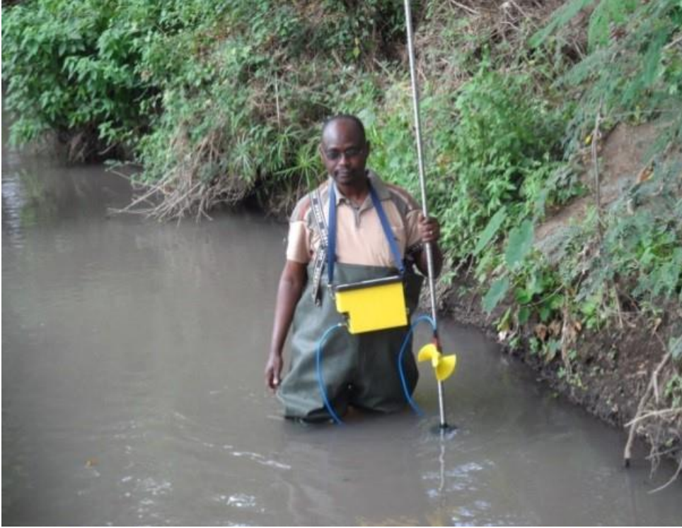
Figure 4: Water flow measurement using current meter
