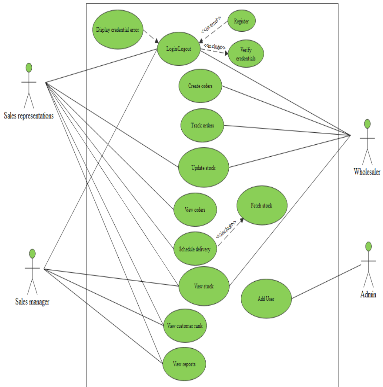
Figure 10: Mobile Application Use Case Diagram
