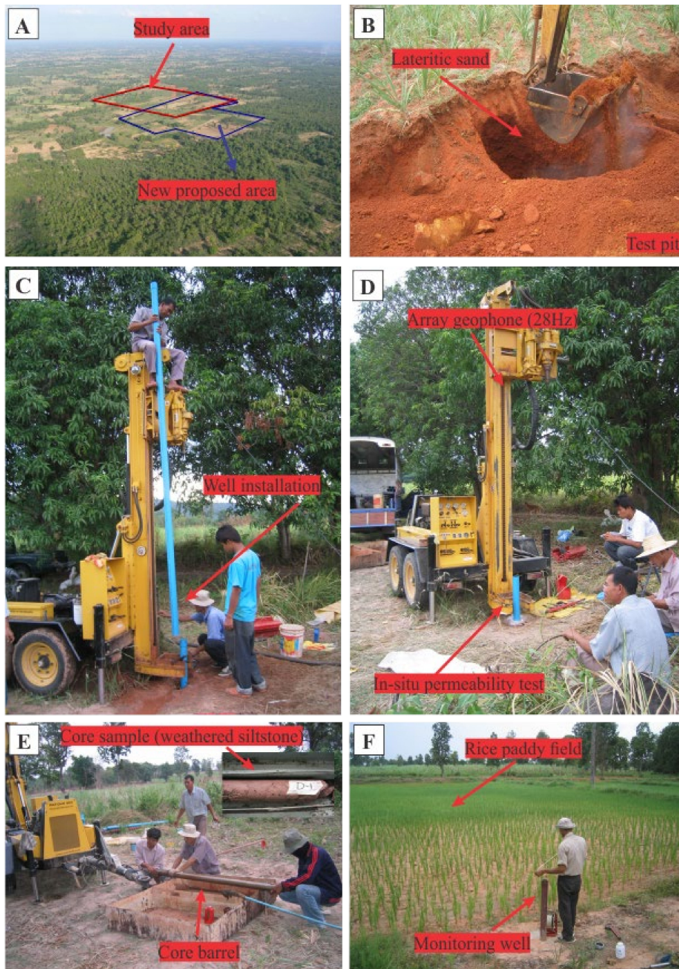
Figure 4. Aerial photos of the study area (A), test pit (B), monitoring well installation (C), in situ permeability test (D), core sample collection (E), and groundwater sampling in the study area (F).
