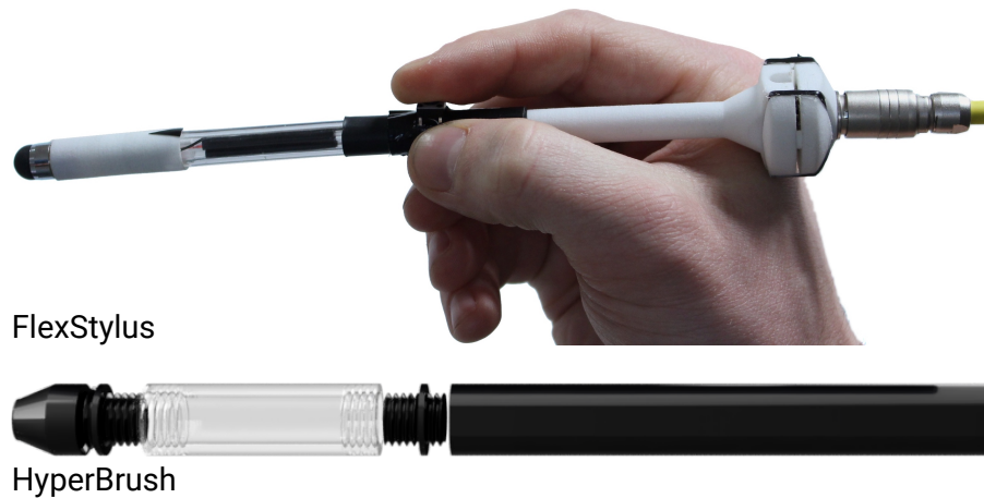
Figure II.5 – Two series of flexible pen prototypes. On the top: FlexStylus with a custom bend sensor made of eroded fiber optics. On the bottom: HyperBrush with a consumer electronics bend sensor, and interchangeable flexible components.
