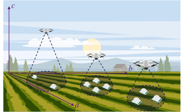
Fig. 1: An example employing 9 nodes and 3 drone positions.
