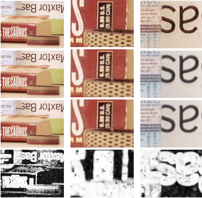
Fig. 12. Image fusion for a real focus sequence obtained with different algorithms. From top to down: first row, Helicon Focus software [24]; second row, 3D EDF algorithm [6]; third row, proposed SAF algorithm; fourth row, \phi_{x,y} .
