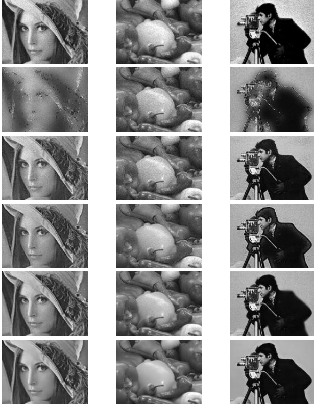
Fig. 9. Image fusion for synthetic focus sequences obtained with different algorithms. From top to bottom: Zerene Stacker [25], Algorithm of Tian, et al. [26], EDF [7], Helicon Focus [24], 3D EDF [6] and proposed SAF algorithm.
