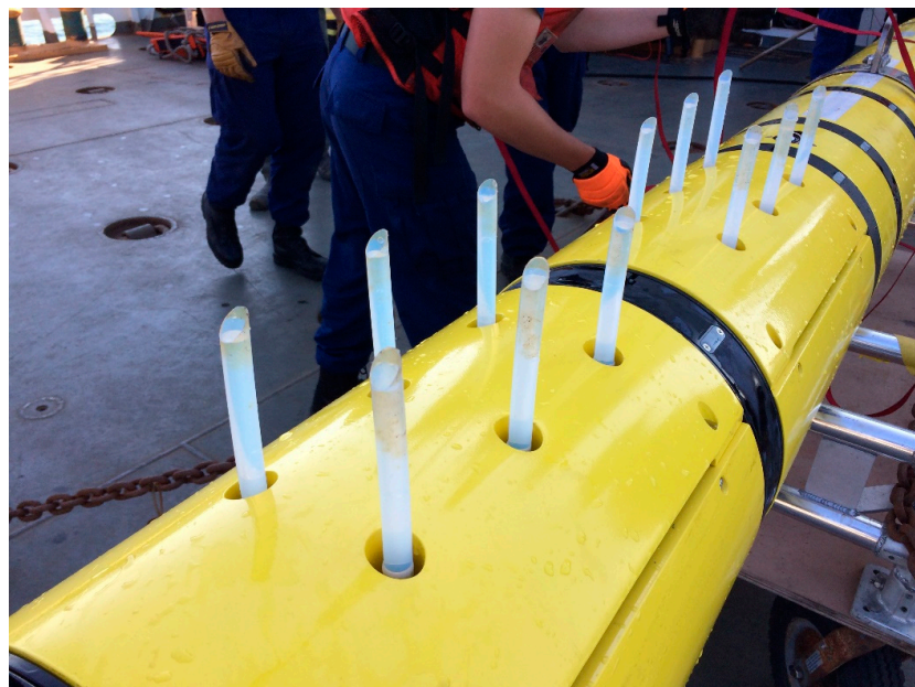
Figure 1. REMUS 600 AUV integrated with the Midwater Oil Sampler.
