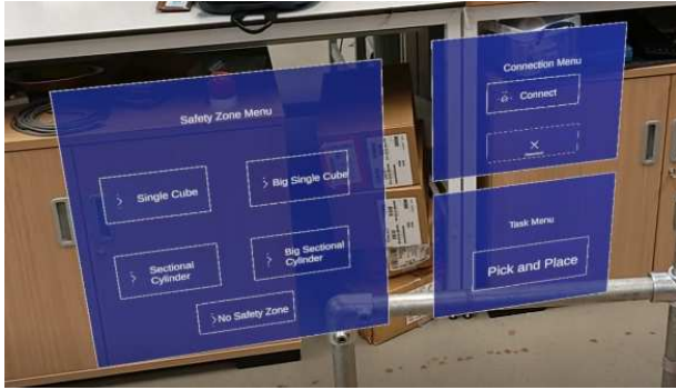
Figure 5: Panel type user interface for HoloLens 2. The safety zones can be configured using the UI.
