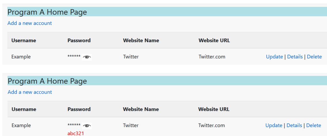
Figure A.3: Main page of program A which shows a stored account. The page shows website name/URL, username and password as asterisk. The second screenshot shows the password when a user puts the cursor on the eye icon.
