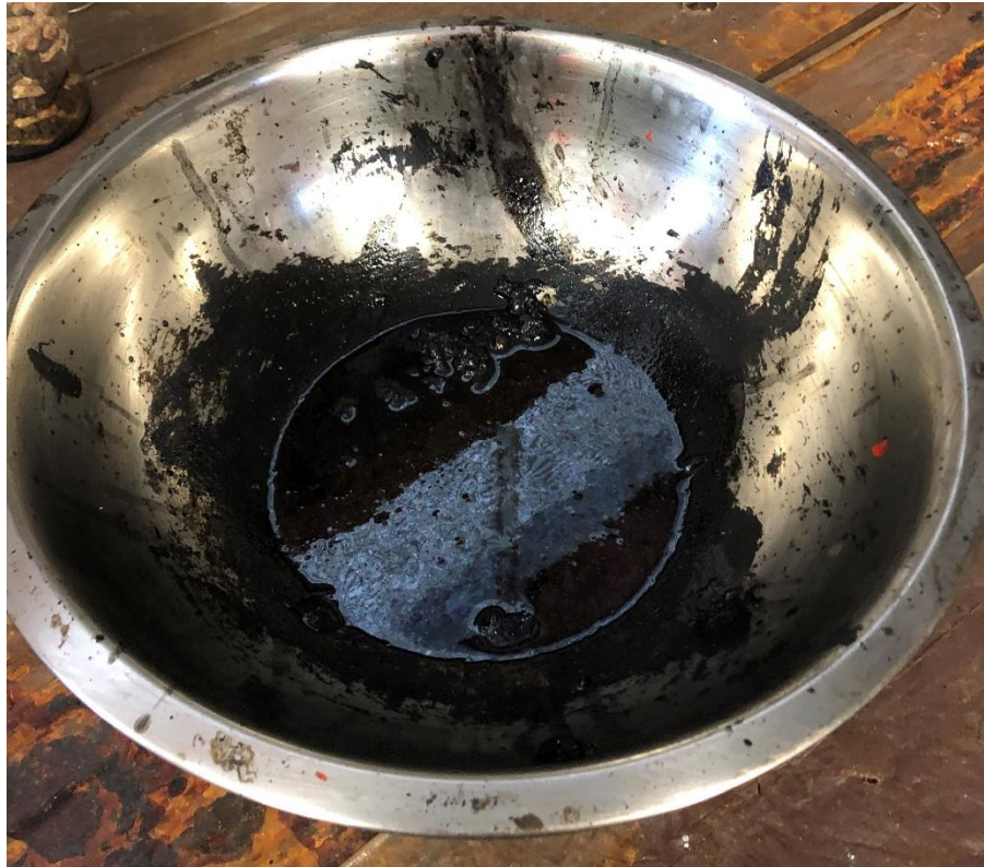
Figure 4.10 Image of tar captured from the downdraft gasification system
