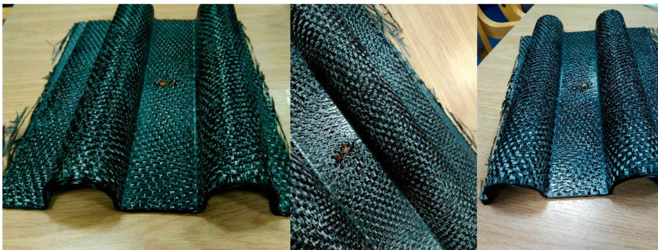
Figure 3. Images of re-pressed preform using an omega shaped tool.
