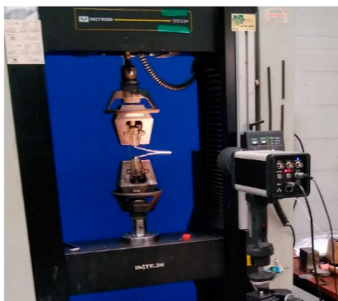
Figure 9. Mode 1 machine + camera setup.
