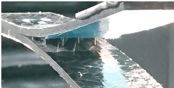
Figure 14. Bridging observed with Kevlar samples.
