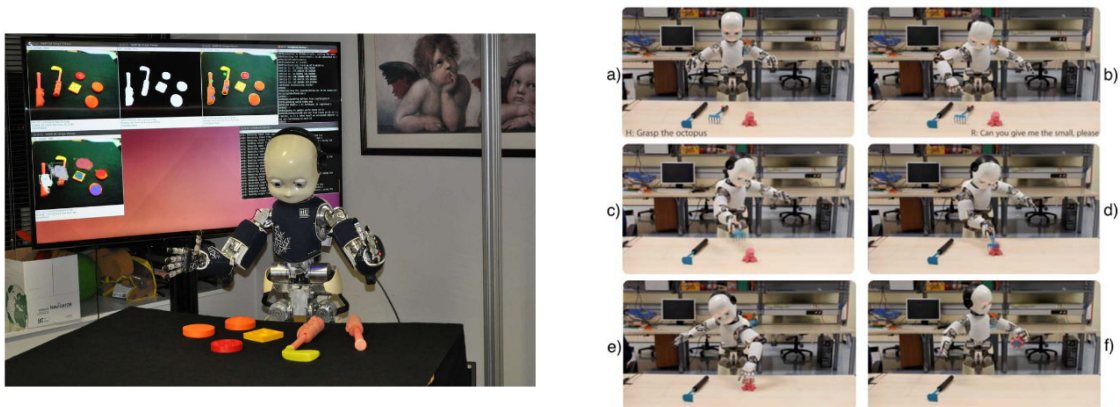
Figure 2.2: Images show a typical scenario for relational affordance detection for tool usage learning. Image on the left shows the visual perception system (i.e. object segmentation and tracking). Image on the right shows an interaction example where a robot is asked to grasp an object. The robot has learned that a particular tool allows him to bring the target closer. Images taken from [78] and [72] respectively.
