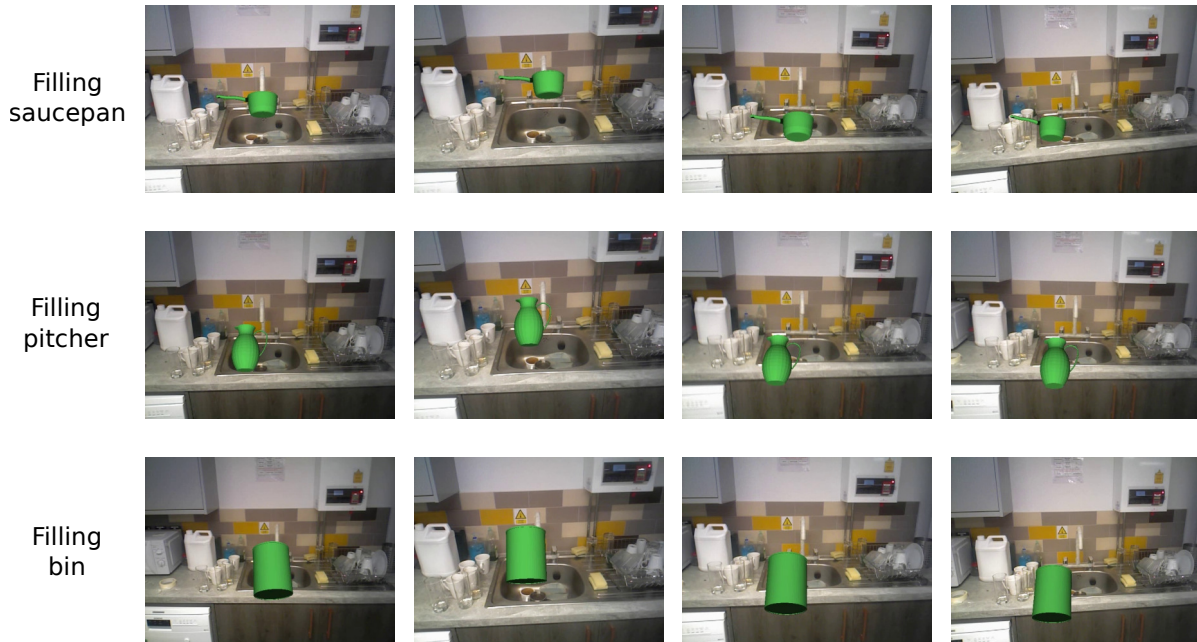
Figure 6.10: Affordance lantern example predictions for Filling affordances. Notice that the tilted pose of the query-objects is due to errors in the camera pose estimates, despite the noisy camera pose estimates, the affordances are correctly predicted in the tap.
