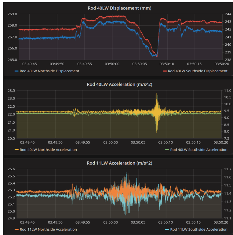
FIGURE 2.4. The SHM dashboard produced from trial 1. Acceleration and displacement data captured by the six sensors in the WSN: the CSB’s structural response to a single vehicle entering the bridge at the Clifton is displayed. Figure reproduced from Gunner et al. [94].
