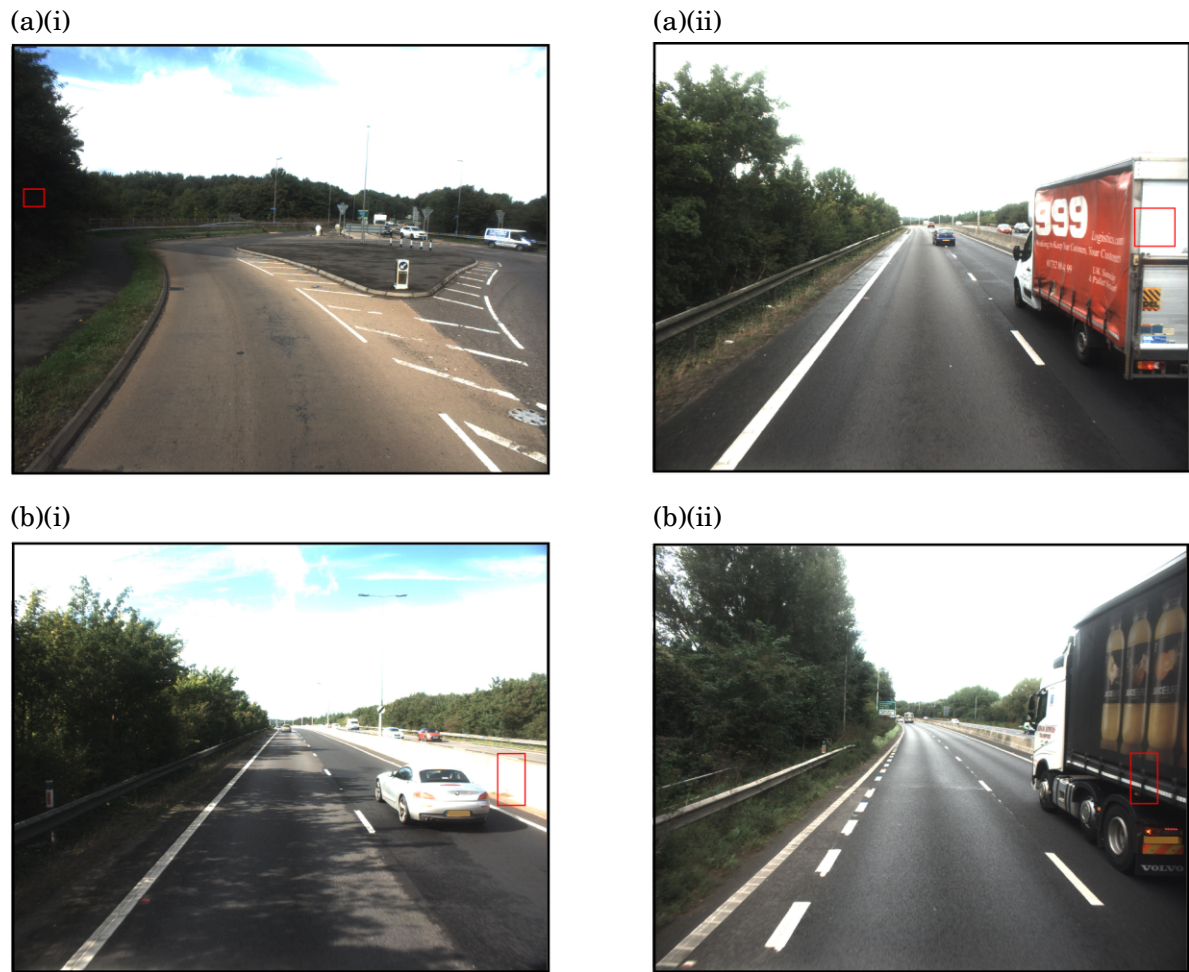
FIGURE 3.15. (a) Traffic signs and (b) reference markers that are correctly recorded in the inventory but are identified by the system for further manual inspection. The assets in the (i) panels are incorrectly classified by the CNN whereas the assets in (ii) panels are impeded.
