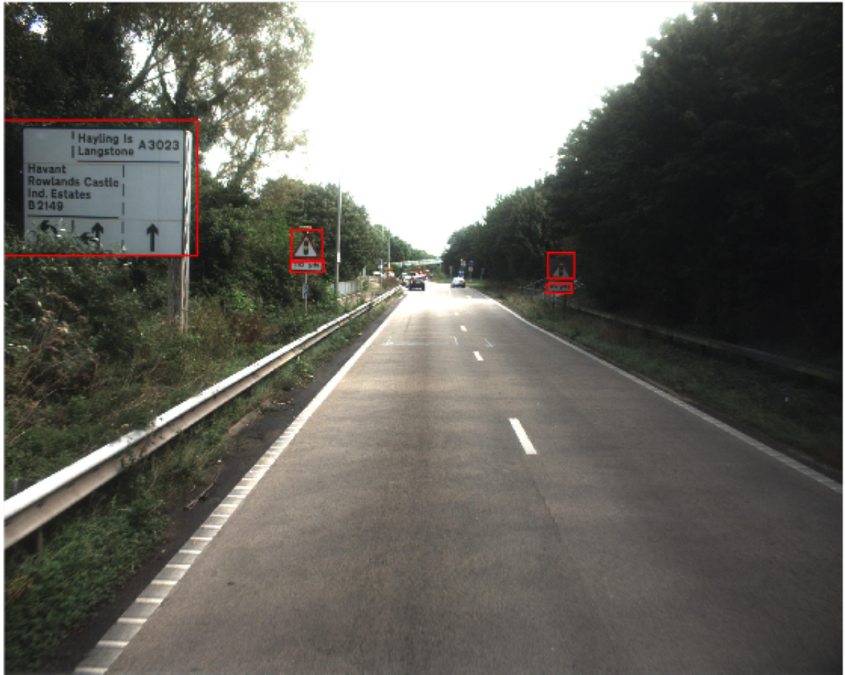
FIGURE 3.9. Bounding boxes of five traffic signs constructed by the perimeter around the pixel coordinates computed by Equation 3.5 for the entire position of the asset relative to the vehicle. The asset width and height are extended by 0.15 m in each direction to ensure the assets appear within the computed bounding boxes.
