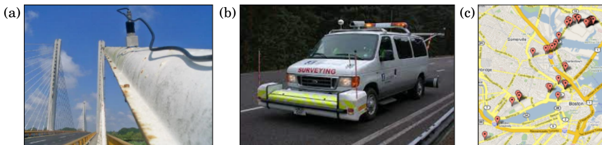
FIGURE 1.2. Sensing modes in transportation asset management (TAM). (a) Fixed accelerometer installed onto a bridge. (b) Specialised vehicle used to collect pavement condition data on a drive-by remote survey. (c) Potholes detected ad-hoc by a fleet of taxis in Boston. Panels (a), (b), and (c) are respectively reproduced from Carrión-Viramontes et al. [39], Highways England [115], and Eriksson et al. [67]
