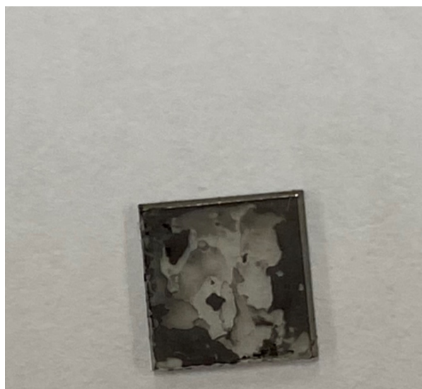
FIGURE 7.22. Photo of SN1707, poly-crystalline U_3Si_2 , after exposure to 0.1 mol. H_2O_2 for 8100s. Data from SN1707.
