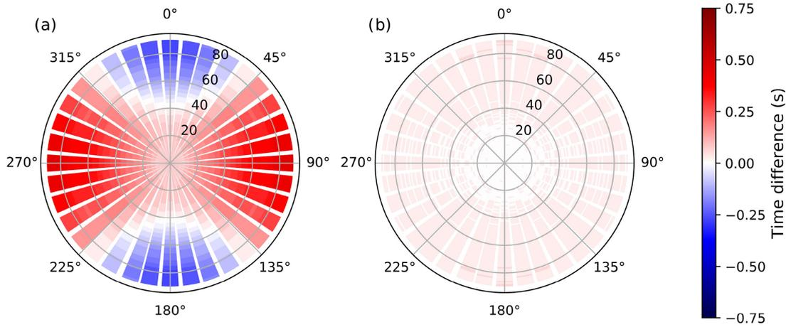
**Figure 2.** Rose diagrams showing the magnitude of the time difference between the elliptical and spherical SPECFEM3D synthetics for (a) uncorrected and (b) corrected  $P$  waveforms. The angle from the centre point is azimuth from the source and the radius is epicentral distance from the source. The residual once corrected is no more than 0.05 s at all distances and azimuths.
