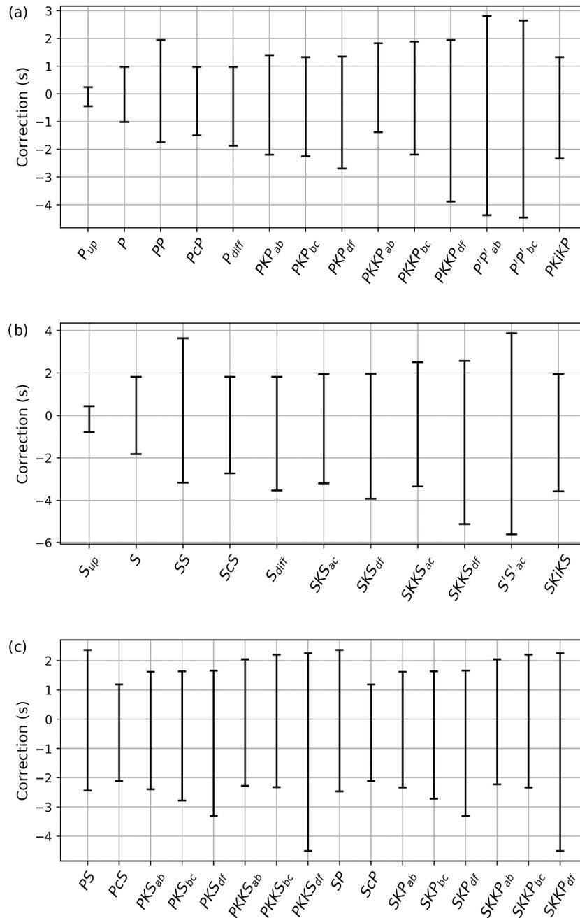
**Figure 3.** Minimum and maximum ellipticity corrections in seconds for commonly used seismic phases.  $P$  phases are shown in (a),  $S$  phases in (b) and converted phases in (c). Tabulated values can be found in Supporting Information Section S3. Corrections for depth phases can also be calculated but are not shown here.
