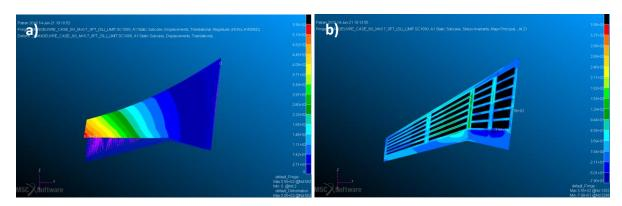
Figure 3: Static aeroelastic response for subcase 1000, a) deformation, b) stress.
