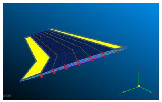
Figure 1: Structural FE model of the combat aircraft wing.
