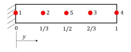
Figure 7: Control points along span of the representative wing.
