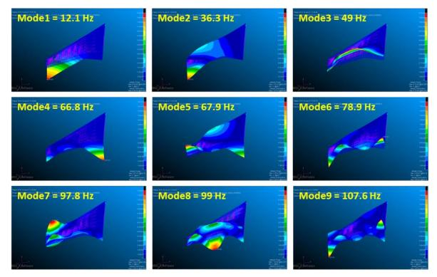
Figure 6: Modal analysis of updated FE model with "0" degree UD angle orientation.
