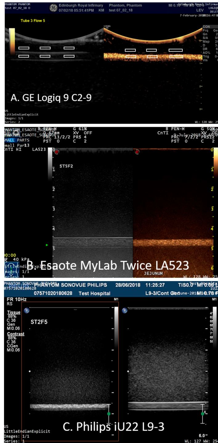
Figure 3. Images acquired from 1.6 mm tubing (A) 1 cm depth SonoVue-filled tube imaged using the GE Logiq9 C2-9 transducer with ROIs highlighted; (B) 5 cm depth SonoVue-filled tube imaged using an Esaote MyLab Twice LA523 and (C) 8 cm depth DEFINITY ® -filled tube using a Philips iU22 L9-3.
