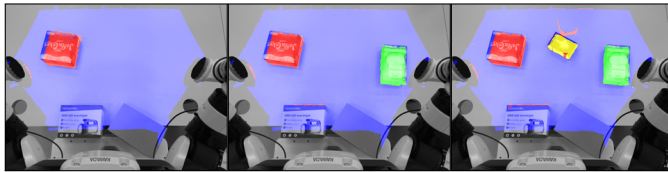
Fig. 8: Segmentation of multiple static objects (red, green, yellow) that are slid by a human on a table one-by-one.
