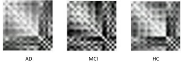
Figure 1. Greyscale 21x21-pixel images (not to scale) representing the correlation matrix computed across all channels from 5s data epochs for one subject from each class.
