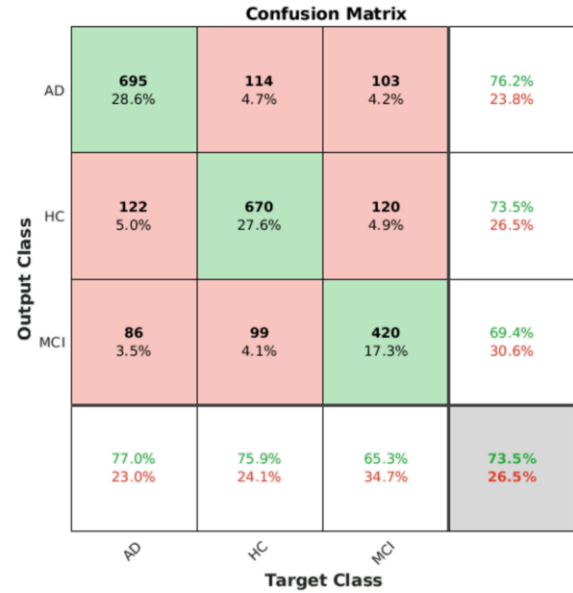
Figure 4. Confusion matrix for the best performing epoch length trials (10s) when images derived from dLZC between electrodes were used as the model input to AlexNet.
