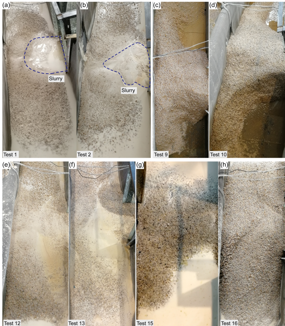
Fig. 9. Deposition morphology of selected experimental debris flows. (a, b) The depositions of flows without entrainment in tests 1 and 2 take the form of typical alluvial fan compressed by the opposite sidewall of the lateral flume. Slurry containing fine components is deposited in the dashed box. (c, d) Deposit lobes of FEC in tests 9 and 10. (e, f) Deposit lobes of FEW in tests 12 and 13. (g, h) Deposit lobes of FEC in tests 15 and 16. The tributary exit is on the right of each picture and the opposite sidewall of the lateral flume is on the left.
