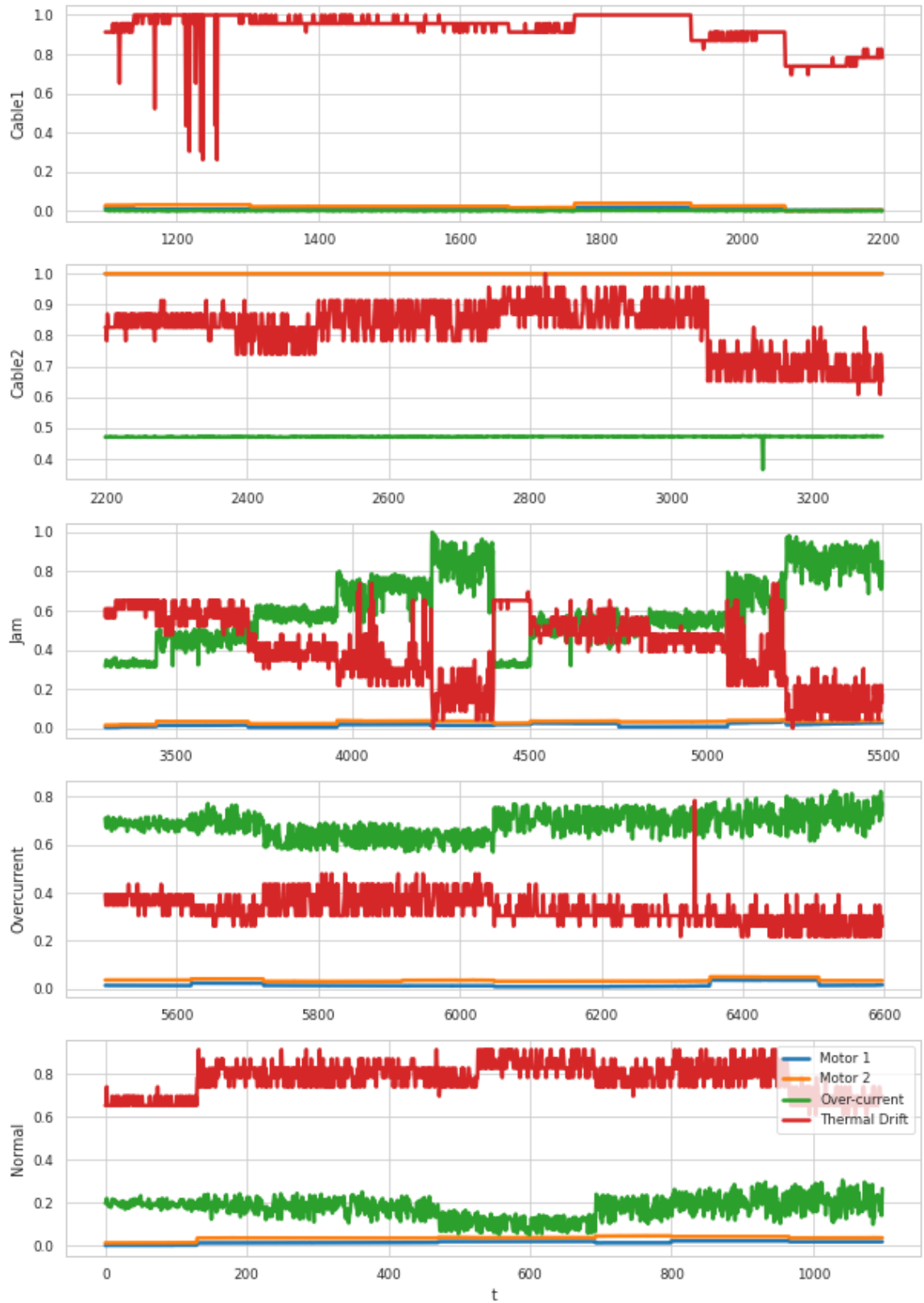
Figure 4.2: Sensor plots per class. Each row of plots show the collective sensor behaviour for each fault class. Each sensor is assigned a color. Output for Motor 1 is blue, output for Motor 2 is orange, Current is green, and Thermal Drift is red. The most descriptive sensor readings correspond to Current and Thermal Drift.
