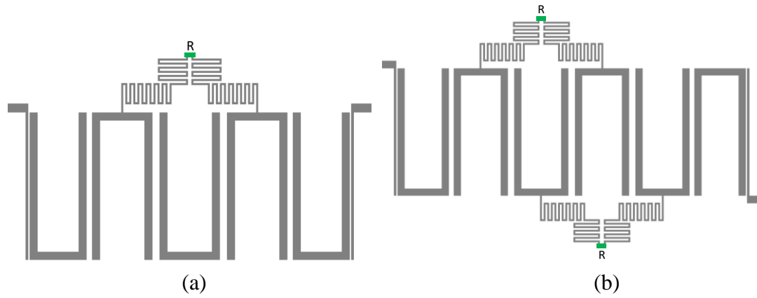
Figure 4.18 Layout of lossy filter implemented as (a) 5 in-line coupled hairpin resonators and (b) 6 in-line coupled hairpin resonators.
