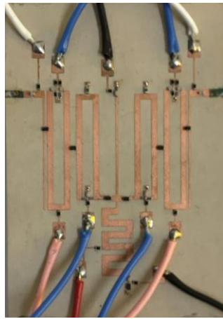
Figure 4.9 Fabrication of the tunable filter
