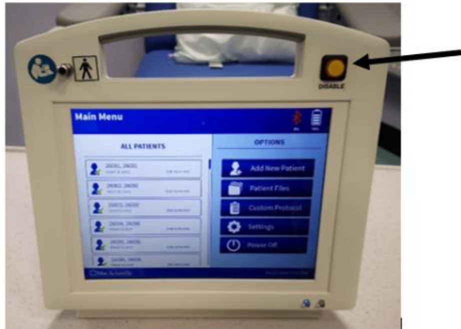
Figure 7b.1 RBB pump showing the DISABLE button in the top right-hand corner. The machine's pneumatic components are only operational if the button is depressed (as per photo).
