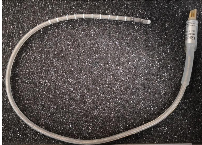
Figure 1.7 Bipolar ring electrode mounted onto a flexible catheter (Gaeltech, Isle of Skye, UK). White, horizontal markings indicate 1 cm intervals from the centre of the two electrodes.
