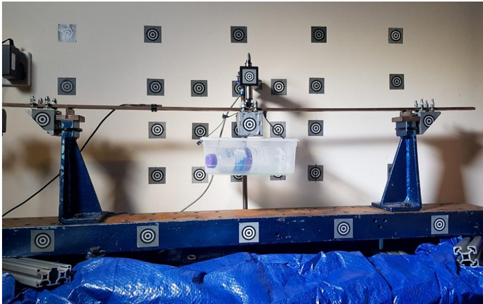
Figure 1: Experimental structure: “Copper bridge”.
