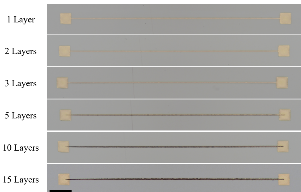
Figure 6-20 Printed line electrodes with various printing layers on the Z10 substrate at the drop spacing of 4 \mu\text{m} and printing velocity of 2 \text{ mms}^{-1} . The scale bar is 200 \mu\text{m} .
