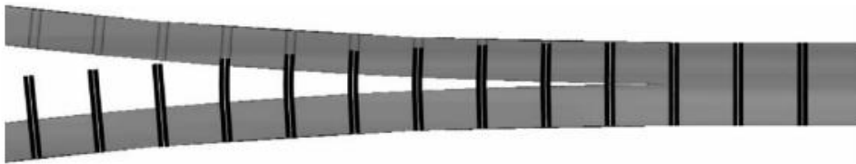
Figure 2.4 Schematic demonstrating the bridging effect of z-pins during steady state crack propagation [69].
