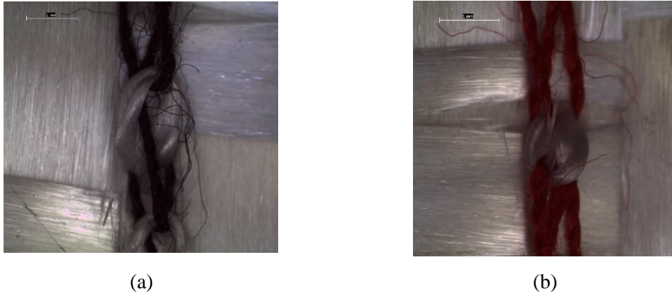
Figure 6.1 Optical micrographs of the junction positions for stitched preforms; (a) fabric type 2; (b) fabric type 3.
