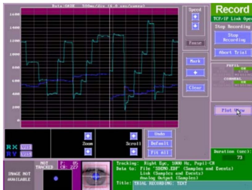
Figure 5.6: Screenshot of the EyeLink record screen. The trace of the participant's gaze coordinates is displayed in real-time. The lower camera image shows the pupil centre crosshairs and CR centre crosshairs. The box on the right signals the tracking status. Image taken from SR Research Ltd (2009).
