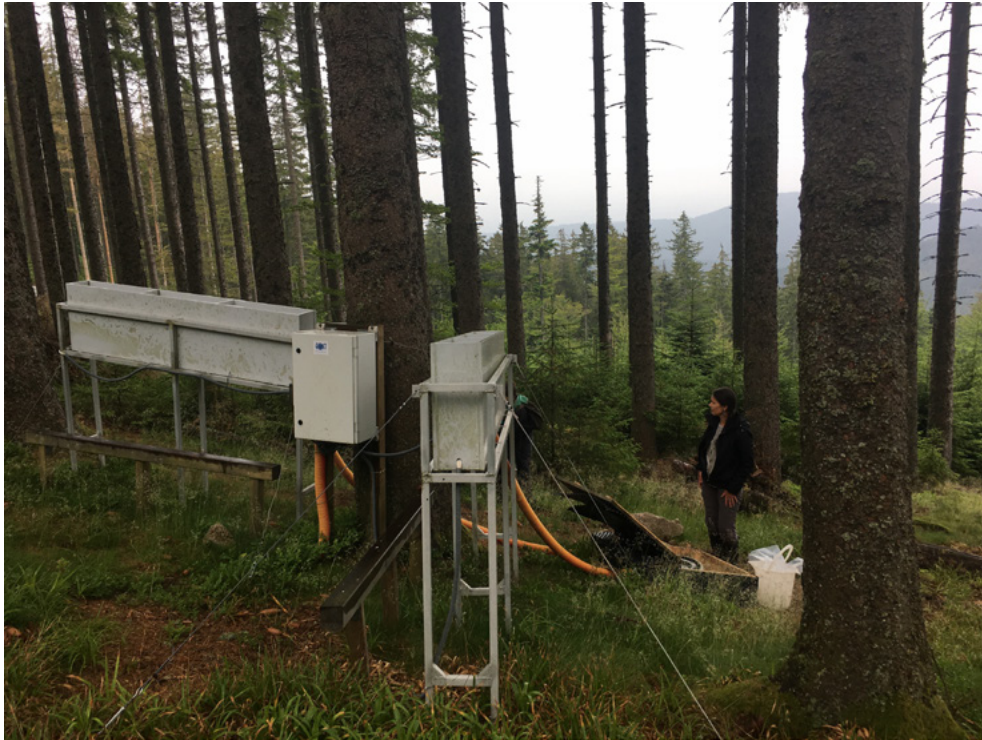
Fig.67. Gutters collecting rainwater under the trees
