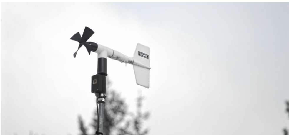
Fig.75. The anemometre Monitoring of wind strength and direction. Video still Sonia Levy.
