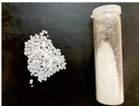
Figure 3. 11 White virgin HDPE pellets of HMA018 before (left) and after (right) cryogenic milling at 25 Hz.
