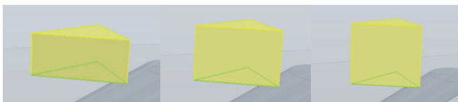
Figure 2 Prism-shaped VG: (a) 0.005m, (b) 0.0075m, (c) 0.01m
