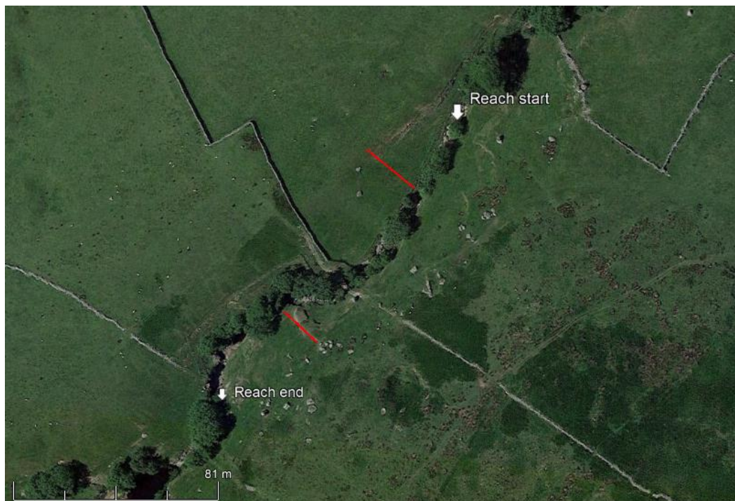
Figure 4-4: Screen grab from GE TM showing reach SP003. Red lines represent the horizontal limit to which a 1m change in elevation data, using the cursor point as an indicator, was recorded.
