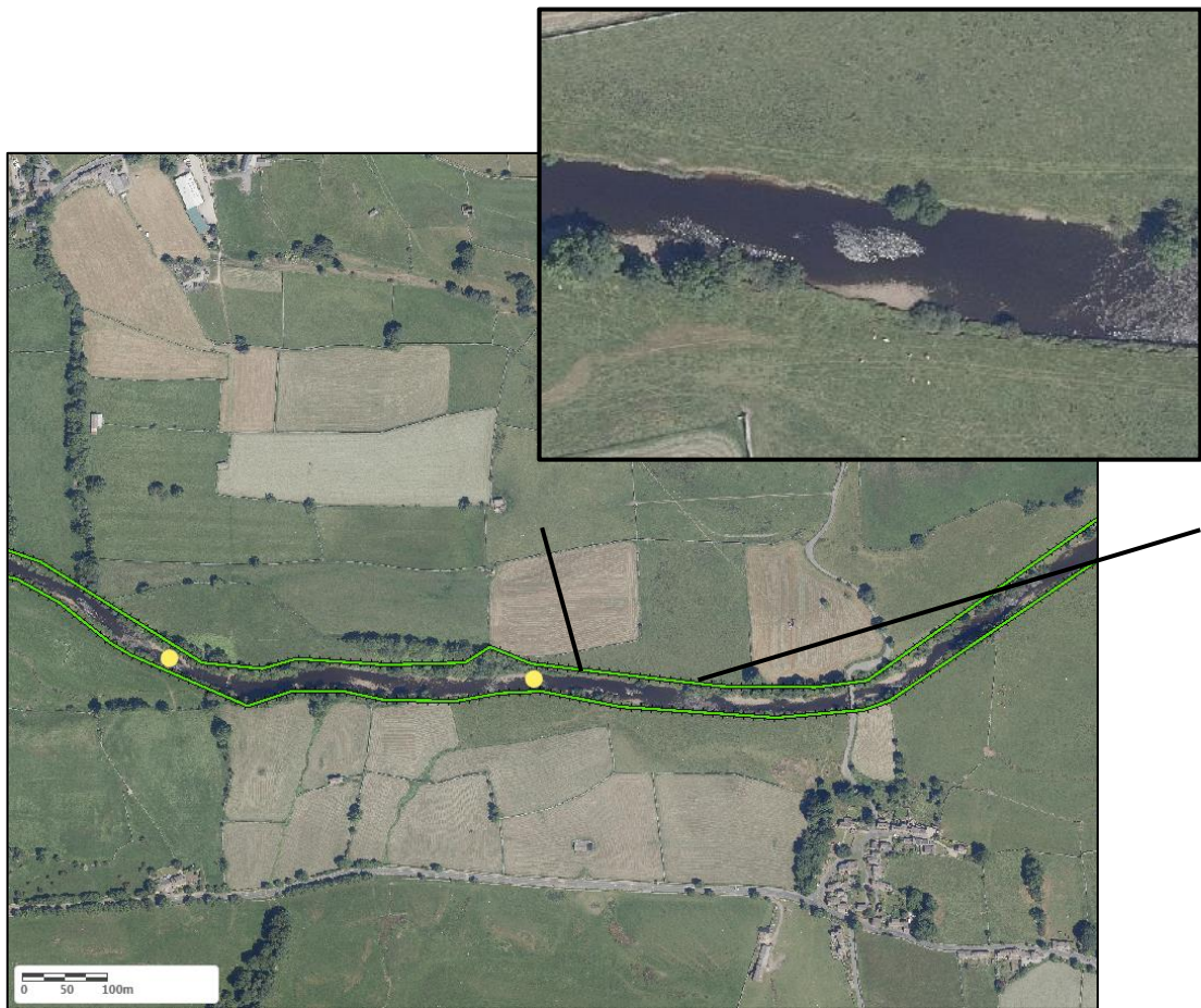
Figure 5-11 Aerial image of River Ure showing EA AIMS embankment dataset whereby embankments are present along both banks. Inset demonstrates that these are not clearly visible in GE imagery,
