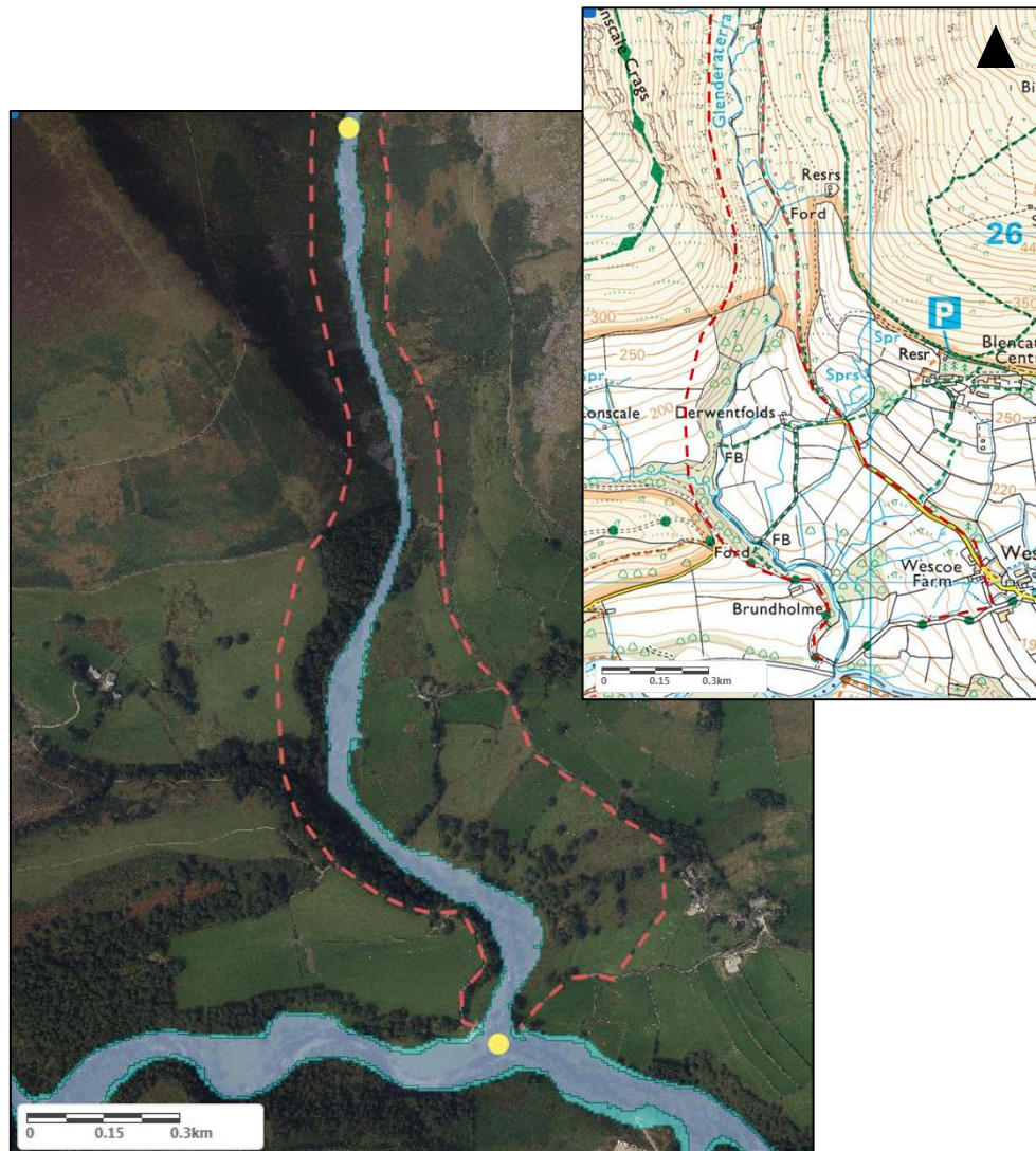
Figure 5-9 Example of manually delineated river corridor width (red dash line) for Glenderaterra Beck, Cumbria study site (indicative river types B and C)
