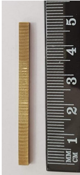
Figure 10. Machined copper strip used in the experiment.
