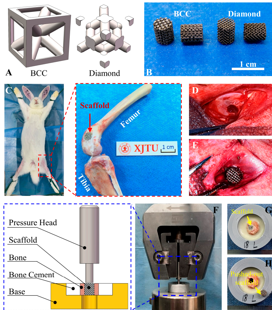
Figure 1. Fabrication and animal experiment of AM scaffolds. (A) RVEs of BCC and diamond porous architecture. (B) Photographs of the scaffolds. (C) The location of the implanted scaffolds. Intraoperative photographs of (D) bone defect and (E) implanted scaffolds. (F) Push-out test of the scaffolds. (G) The scaffolds in the surrounding bone. (H) Pushed-out scaffolds.
