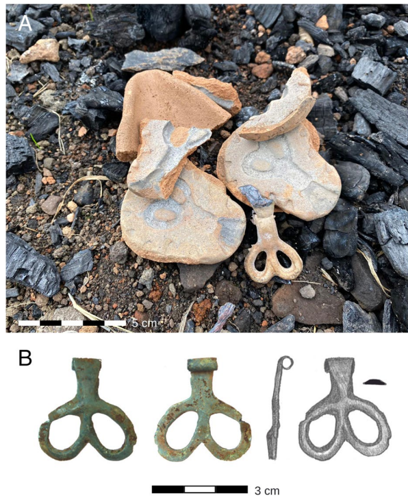
Fig. 16 A Bi-valve mould made and used during experimental tests with cast bronze pendant. B Bronze pendant recovered from Cx. 236 at Şagu (after Sava et al., 2011, p. 51, Fig. 9.1)
