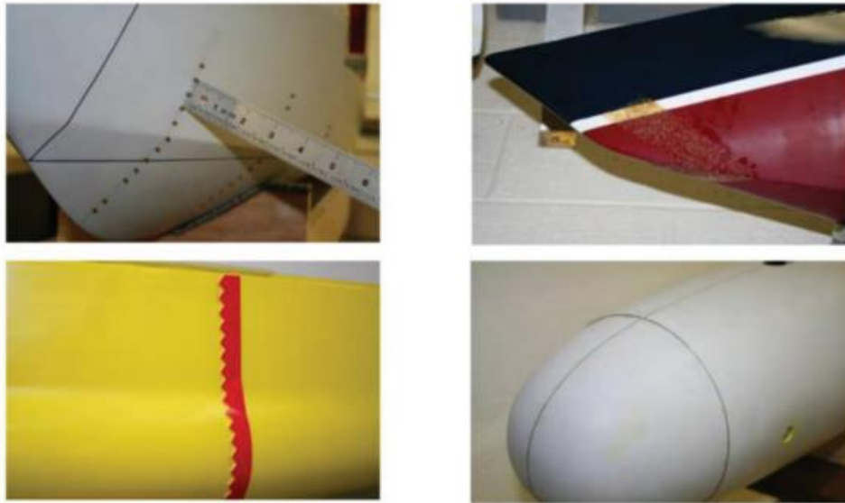
Figure 8: Types of turbulence stimulation devices, clockwise from top left: studs, sand strip, trip wire, hama strips [Murphy 2010].
