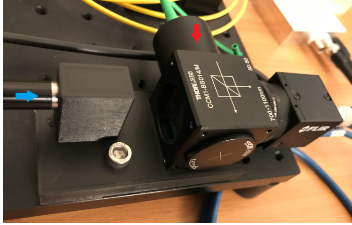
Figure 4.3: CAD designed and 3D-printed off-axis interferometry mount (as delineated by the red dashed rectangle in Figure 3.3). The reference arm (from top) is mounted to the beamsplitter via a lens tube (red arrow) and an externally threaded fibre adapter. This arrangement allows the observation distance of the reference arm to be adjusted to match that of the sample arm (from left, blue arrow), which is a requirement of lensless Fourier holography. N.B. A full system diagram is shown in Figure 3.3.
