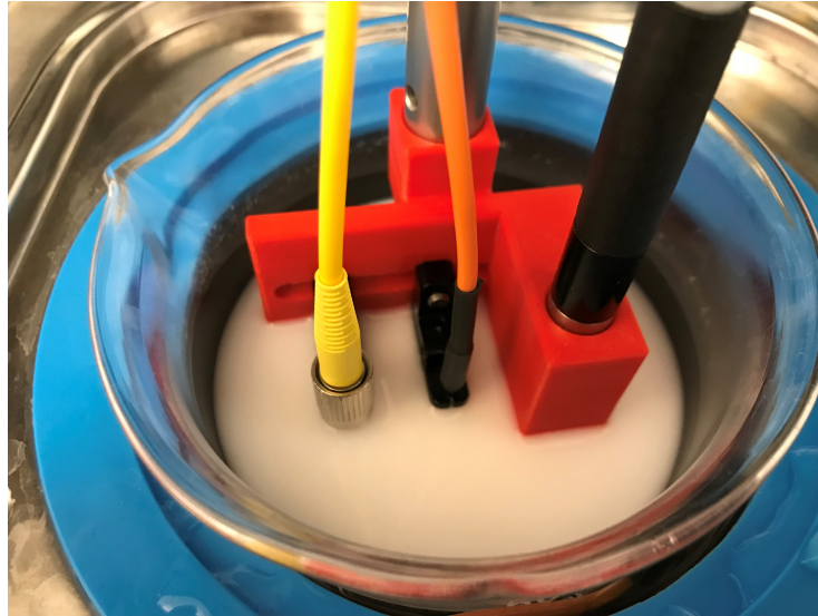
Figure 4.8: Semi-infinite reflection mode geometry used for absolute validation experiments. From left, single-mode detection fibre, multimode source fibre, and LLG, coupled to the intralipid phantom using a custom designed and 3D printed probe.
