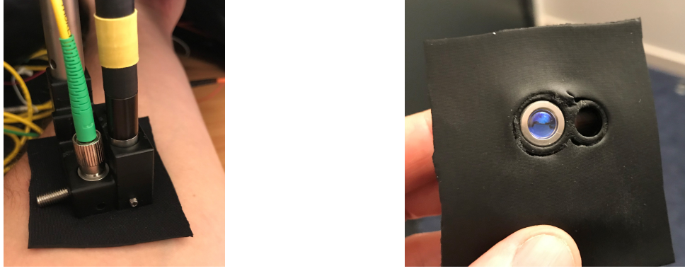
Figure 4.15: Top (left), and underside (right) views of a 3D printed in vivo probe with an SDS distance of 11.3 mm.
