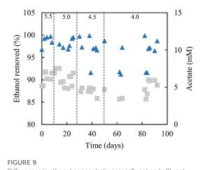
Differences in ethanol concentrations in influent and effluent liquors ( $\blacktriangle$ ), and concentrations of acetate/acetic acid in effluent liquors ( $\blacksquare$ ), during tests carried out with the sulfidogenic bioreactor using ethanol as the main electron donor. Samples were not analysed in the intervals between days 50–62 and days 64–82.
