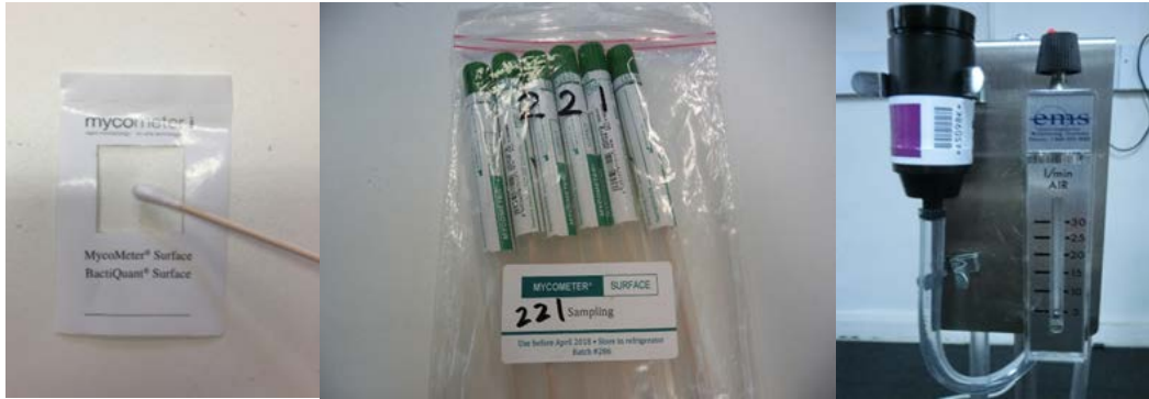
Figure 2: (left to right) Surface sampling, swabs collected from a test room and air sampling (courtesy of Ms Yinzi Chen)
