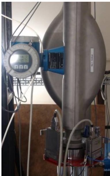
Fig. 2. Coriolis mass flowmeter installed on the vertical section of the experimental rig.
