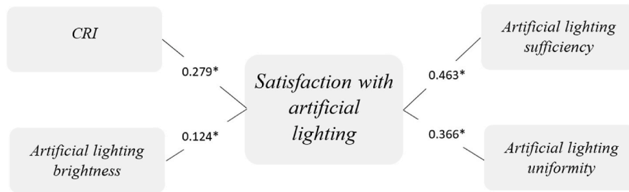
Fig. 8. Diagram showing the correlations for satisfaction with artificial lighting regardless of country (all of the correlation coefficient values shown in the figure are statistically significant* for p < 0.01 ; [31,32]).
