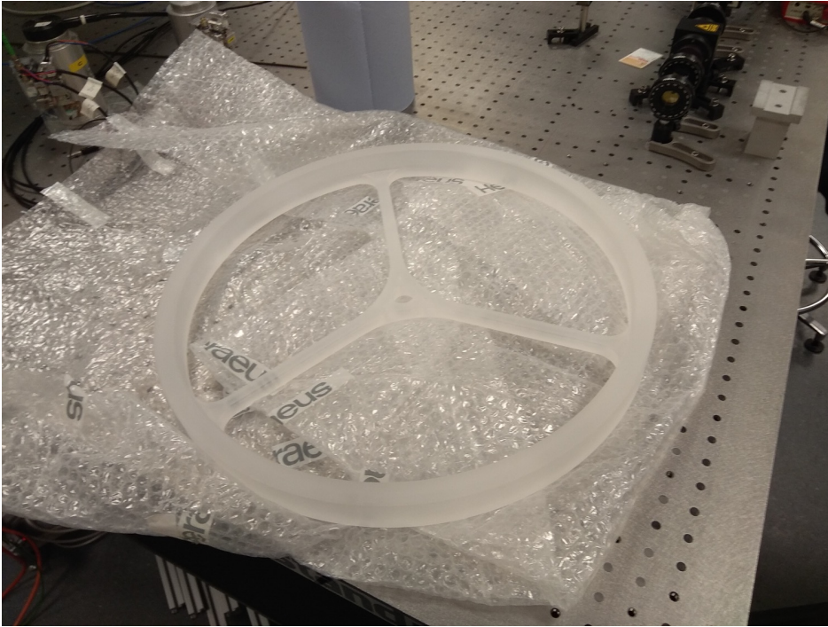
FIGURE 4.10: Photograph of one of the manufactured fused silica test masses.
