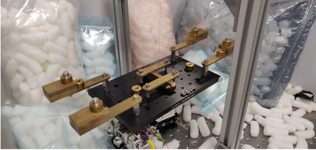
FIGURE 4.1: Picture of the isolated metallic prototype with an interferometric sensor.
