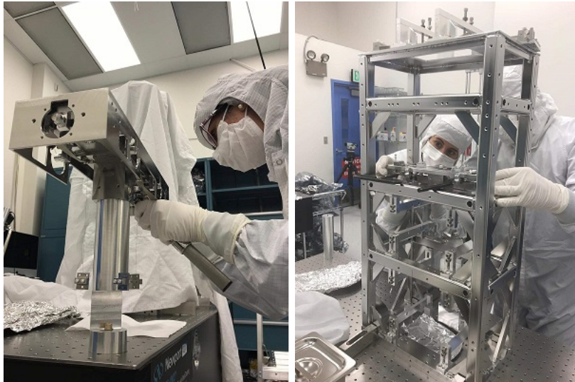
Figure A.3.: Mounting the wires for the test mass suspension on their support. Right: Jeff and I while installing the wire support into the suspension cage.
