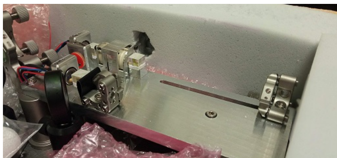
Figure 6.8.: Photo of one of the HoQIs built for the laser stabilization experiment.
