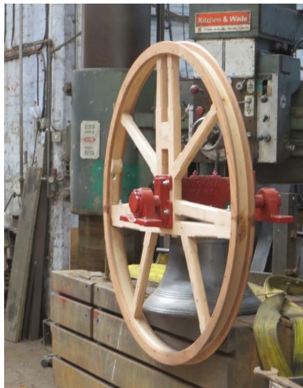
Figure 4-5: Construction of full bell wheel at Taylor's Bell Foundry, Loughborough
