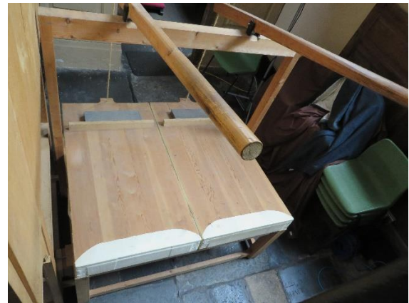
Figure 4-8: The bellows with handles which are pulled in turn to inflate the organ
