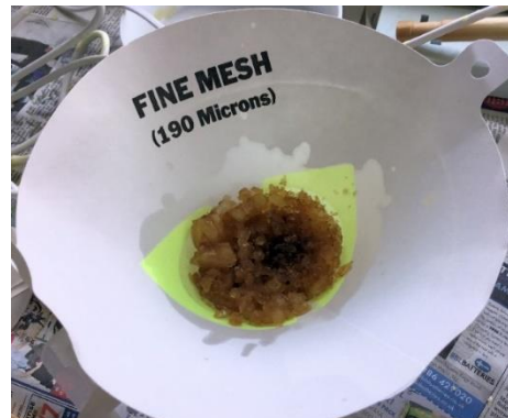
Figure 4: Filtering the mixture to produce tallow
