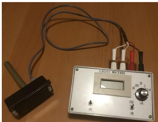
Figure 8: Light meter control unit and sensor
