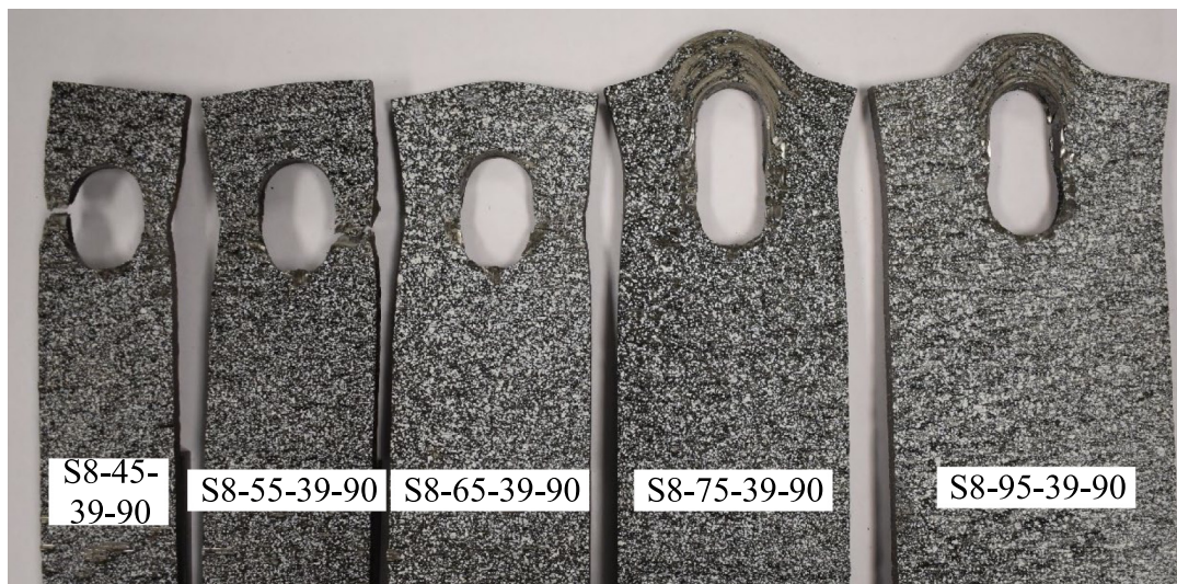
Fig. 16. Failure mode transition from net section tension to end-splitting and shear-out failure.
