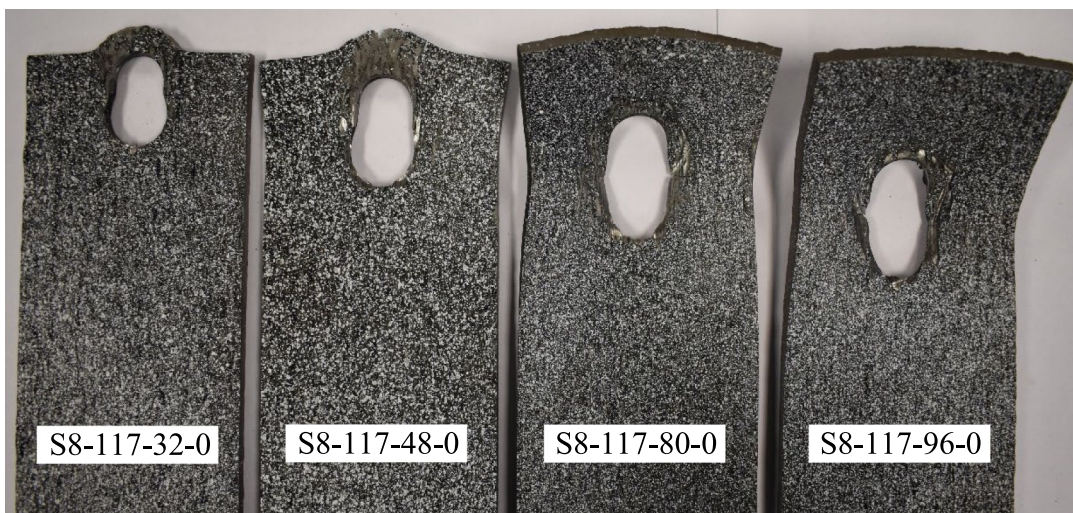
Fig. 17. Failure mode transition from shear-out to end-splitting and localised tearing failure.
