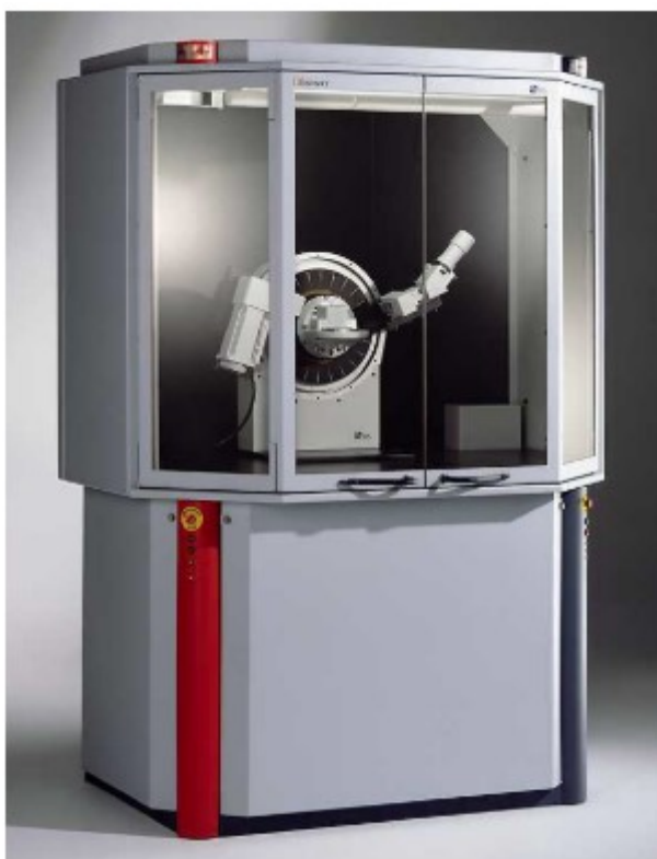
Figure 3.1 A PXRD (Bruker D8 Advance) showing the goniometer and its drives inside the cabinet. 126
