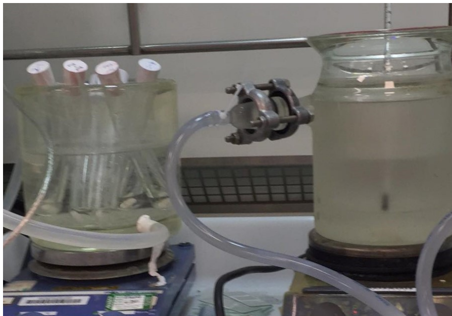
Figure 6.2 Experimental set up for induction time measurement in the lab
